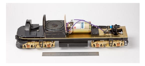
The vertical, rounded baffles help keep the enclosure in place during transportation, and pinch-off the motor cavity to diminish the body resonance. The basswood enclosure is stuffed with ordinary fiberglass house insulation. The speaker and wire outlets are sealed airtight with silicone caulk to prevent back pressure from leaking out and canceling some of the bass notes.
