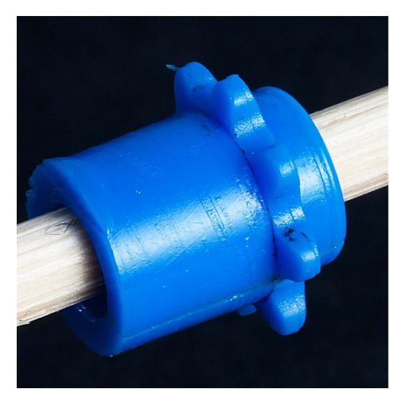
Notice that the injection mold was made in two halves, with the parting line running through the top of the teeth. The two halves are reasonably-well registered with each other. For some reason, one side of the tooth has a shallow angle and the other side a much steeper angle. The crack from hoop stress is visible near the bottom of the photo.
