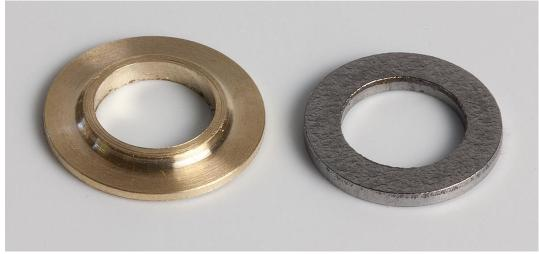
When installed on the shaft, the new shoulder washer affords more than adequate clearance for the chain, about 0.020" shoulder depth, and with far less radial slop than the OEM washer.
