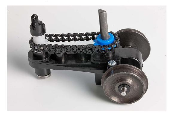
My first peek at it with an Optivisor revealed that the shape of the replacement sprocket teeth had a very different profile compared to the original, and that the replacements were malformed. First, a reference photo of the cracked original.
