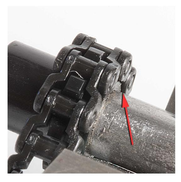
One solution is to make a custom shoulder washer. The nearest larger number drill (in this case, #12) offers a much tighter fit against the shaft and far less wobble. The small diameter faces the sprocket. Once the lathe is set up, you might as well make a big pile of them. This Saturday morning I turned over 30, enough for the P&D drives I have and a few for friends.
