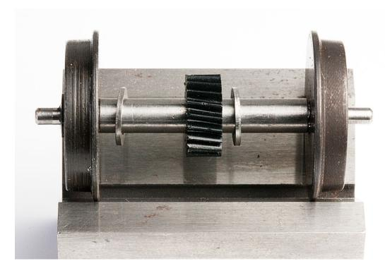
And here is a Northwest Short Line 0.145 tread width replacement, 0.921 diameter and a tread diameter of 0.830. This gives a flange depth of (0.921-0.830)/2= 0.0455. Note that this wheelset was made by the "old" NWSL prior to selling the business to a new owner and it was still in my personal drive rebuilding "stock." I presume the new ones are just as good as the old.
