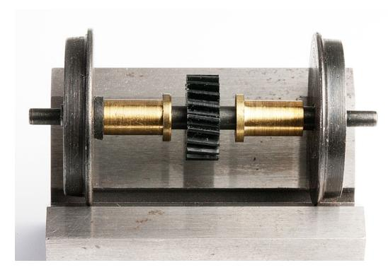
The worm gear seems to have a little bit different tooth profile, but runs just fine in one P&D A unit that I converted about 2002 for running on A&O 1.0. (The worm is the driving gear that looks like a screw.) It seems to have fewer rough edges than the OEM. Also, the shaft has a pair of brass or bronze sleeve bearings to reduce wear on the acetyl gear box cases.
