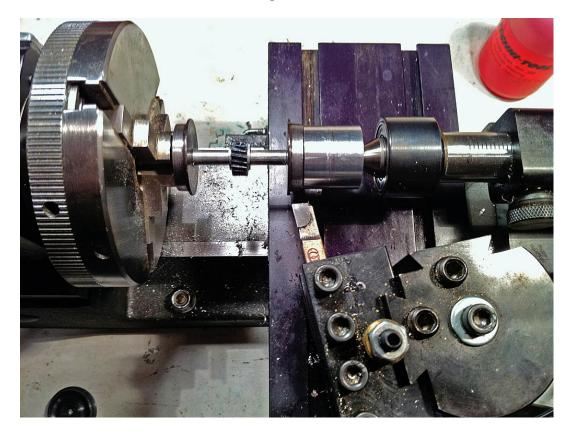
So... now I have another big chore to do! While I have the wheels out of the gear boxes, I will kiss the back of each wheel to smooth out the grooves and knock off the oil finish. That will offer better electrical pickup to wipers.
