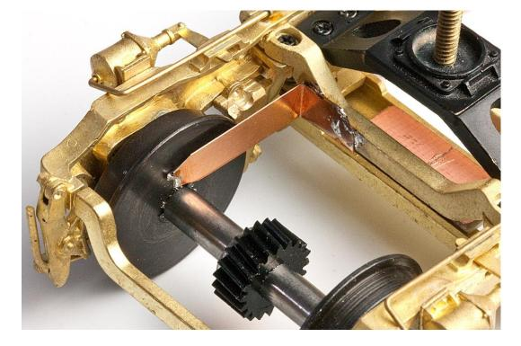
To stop squeaking, drag at the contact point acts in a straight line along the 0.005 phosphor bronze
