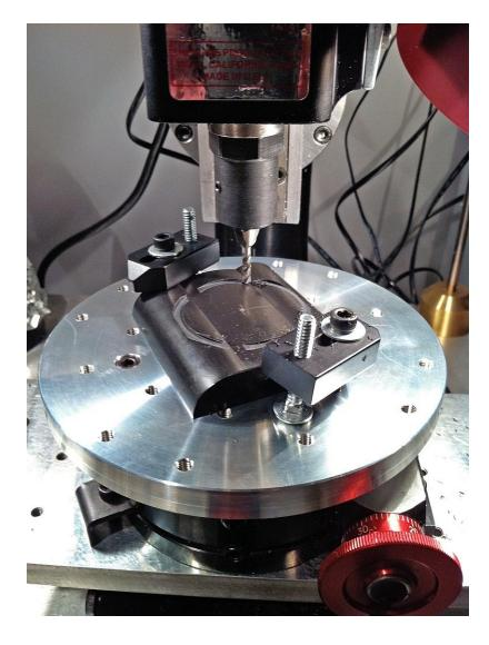
The holes came out fine, with minor flash to clean up. I saved the fuel tanks in case you can find a use for the scrap. (Or was I supposed to cut the tank and scrap the doughnut hole?) Remember that these will now only fit the QSI 2.07 inch High Bass speaker. It is currently the best "rumble machine" I was able to find and fit in the locomotive. The Soundtraxx equalizer can do wonders with this speaker.
