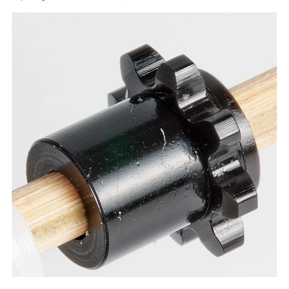
Notice that there is no mismatched mold parting line running through the tooth profile. The teeth are considerably wider than the original P&D sprockets, and this may require more careful alignment with the mating sprocket. When I wrapped chain around the largest sprocket I purchased, there was very little "give" along the axis of the shaft that would allow for misalignment.
