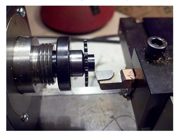
The new 20T sprocket bore is too loose to fit without slipping on the lower P&D drive shaft, so it needs to be pinned in place. I'm drilling for 0.032 diameter brass wire. The blue painter's tape keeps the upper sprocket from flopping around and possibly breaking the carbide drill.
