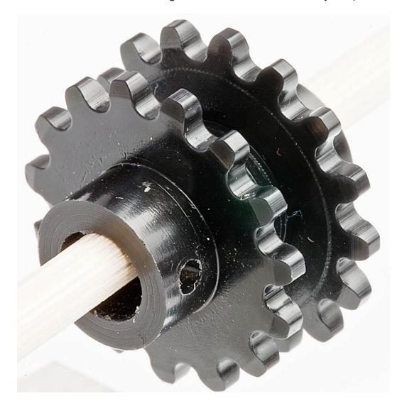
Barely visible is a difference in the root or valley between teeth. It is broader on the ServOLink sprocket. Also the top of the teeth are rounded more on the ServOLink one. Is that the cause? I don't know. But I do know that there is a huge difference in running quality between the two of them. I will donate new sprockets to the cause.
