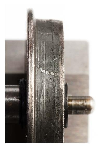
Observe how the crud seems to pack into the depths of the grooves then start to smear across the face of the wheel. Although difficult to see, as it is out-of-focus, the fillet between the flange and tread is much too sharp. This area often had to be cleaned out with a knife. Note that I've increased contrast and heavily sharpened the photo in Photoshop to make the details easier to see. The photo was made with a Canon 100mm L macro lens and a 1 inch extension tube for extra magnification.
