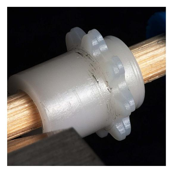
The tooth shape was very different, but notice how the two halves of the mold were not registered with each other. The right half did not center along the bore axis and was shifted quite a ways away from the camera. The chain can not fit smoothly around the entire circumference of the sprocket without binding.
