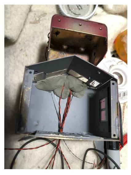
A new hole in the back of the cab, above the simulated control panels, carries 20 wires into the long hood just below the roof. The red and black wires are very flexible ESU 36 AWG wire. The ultra-fine white and gray wires go to pre-wired 0402 red and white LEDs from LEDBaron, a German eBay seller. Each of those LEDs was dipped in ACC then in setting solution for electrical insulation.
