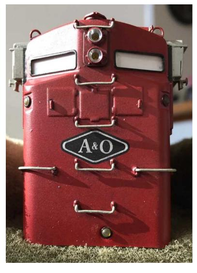
Yes, the upper headlight is loose and has slid outside of its brass investment casting. It will receive additional glue before the rear headlights are also packed in gray clay.
