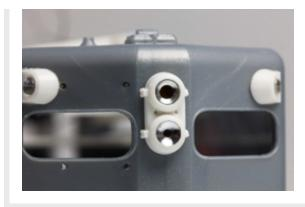
Alternatively NCE's warm white 3mm LEDs work well. These are available from a number of vendors and come in inexpensive 10-packs. These can be inserted directly into the headlight castings with the LED lens just proud of the outside mounting ring.
