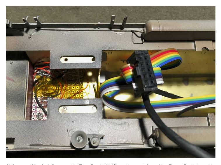
At the rear of the install we see the Tang Band 1925S speaker module and the Power Pack. I need to make the speaker mount more robust; a couple thin strips of double-stick tape are not adequate to hold it in place. A rear PC board that holds the LED resistors is mounted vertically, just to the left of the Power Pack. Both PCBs are mounted with M2 screws into structural supports inside the locomotive. They are not going anywhere.
