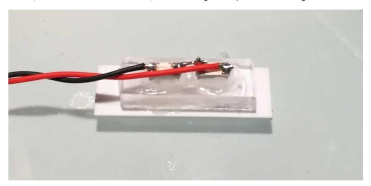
Onto the light pipe two 1206 2700K warm white LEDs from Mouser were glued. The assembly, held down to the work table with tape, offered a perfect platform for attaching wires. These two LEDs, each of which drops about 3 Volts, are hooked in series. Then each end's LEDs get wired in parallel, and fed through a single 1K Ohm resistor. There will be plenty of light, and because these LEDs came from the same reel (batch), and were made by Cree instead of a random Chinese vendor, they
