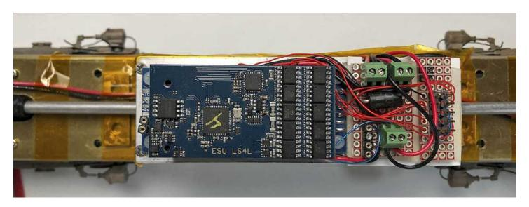
Here's the mating connector and the ribbon cable. One of two hand-wired circuit boards can be seen. This one has the resistors needed to drive the LEDs in the nose of the locomotive. The black thing which seems to come out of the bottom of the 10-pin plug is just a cable for the ESU Maxi keep-alive (Power Pack.)
