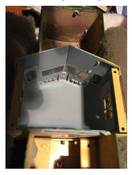
Inside the cab, the only difficulty is that there is are undersize holes on the inside for the headlights. That can be fixed using dental burrs and a die grinder, a/k/a "screaming banshee handmill", a/k/a Dremel or Foredom shaft. I don't advise attempting to drill them out. Don't ask how I know, but something bad can happen.
