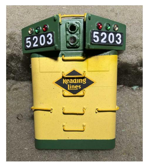
The next photo shows the end of the long hood. I used a "Screaming Banshee Hand Mill" (term learned from Jay Barnaby) with an inverted conical dental burr to grind out a first part of the engineer's side number board and clear out access to the rear headlights.
