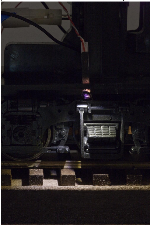
The fixture attaches to a stock Red Caboose chassis and quite nicely lights up the ties as would the prototype. Once trimmed to length, the portion above the frame fits into the cavity under the cab. Obviously another coat of paint will be applied.
