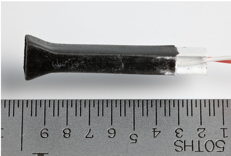
The business end of the light hosts one of the 0603 LEDs.
