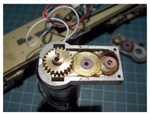
The unit came with an old Sagami motor, probably 5 pole. It had a lot of cogging and the input gear set screw made a nasty burr on the shaft. Cogging primarily happens when the field magnet attracts pole pieces of the armature and causes uneven torque. Skew-wound
