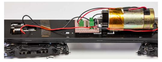
The empty 4 pin gold connector is wired with power on the outside two pins and motor on the inner two. Plugging the mating connector in backwards can cause no harm and only result in swapping the locomotive's running directions.
