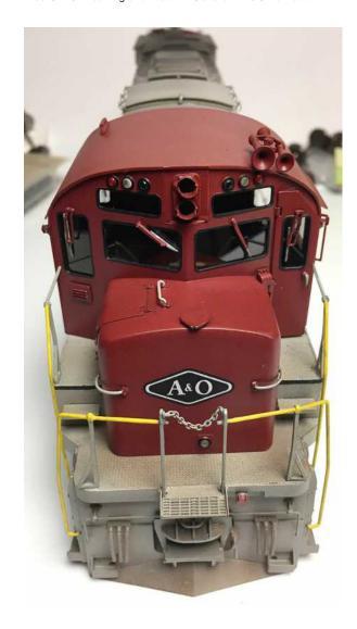
I was originally planning on just lighting the white class lights. But while watching a video review of an HO UP gas turbine model I noticed that the front class lights could be rotated between all 3 colors. How'd they do that? Yesterday I stumbled upon exactly that in a sound schedule for a Loksound V4 645 turbo. This particular file was edited by a good friend for an engine on his layout. Here's a peek at LokProgrammer showing the Class Light "code" in sound slot 10.
