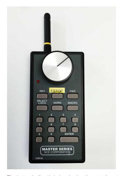
The button is directly below the throttle potentiometer, so it is easy to locate without looking.
