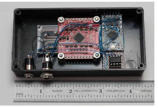
It was not worth etching a circuit board since there is only one extra IC, a Maxim RS485 interface chip. Double-stick tape holds the perforated board and Arduino Pro Mini in place. The large jack receives a 5 volt DC wall wart for power. A 3.5mm stereo jack attaches brings signals
