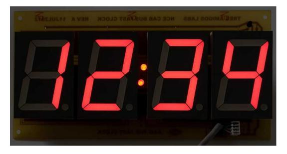
The roughly 4x8 inch board uses an Arduino Pro Mini from Sparkfun in Boulder, CO. There are a few jumpers as this is a home etched single sided board. Source code is only about 100 lines of C++.
