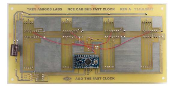
A production run of 5 Rev B clocks begins tomorrow. The only planned changes are the addition of a missing trace and pads for the 1K ohm resistor tacked above the processor. The resistor's only job is to shunt current around the colon LEDs to better match brightness to the LED numeric displays.
