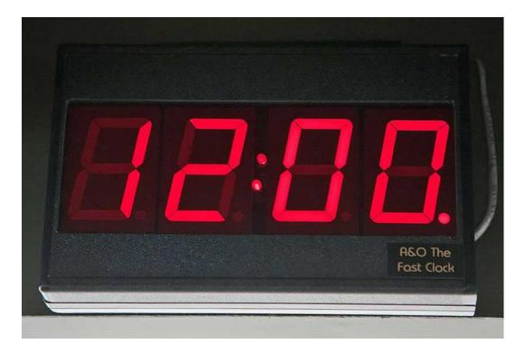
In the photo a single CAT5 cable (to be painted black) exits the right side of the case and disappears through a hole in the valence above the clock. Immediately behind the clock, on the opposite side of the Masonite valence resides a 4 foot fluorescent fixture. Making a cutout through the valence for a RailLogic clock would not be a viable option in this location.
